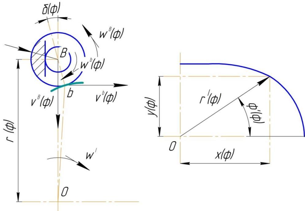
Figure 4. Determining the true ear profile in the Polar (a) and Cartesian coordinate system (b).
