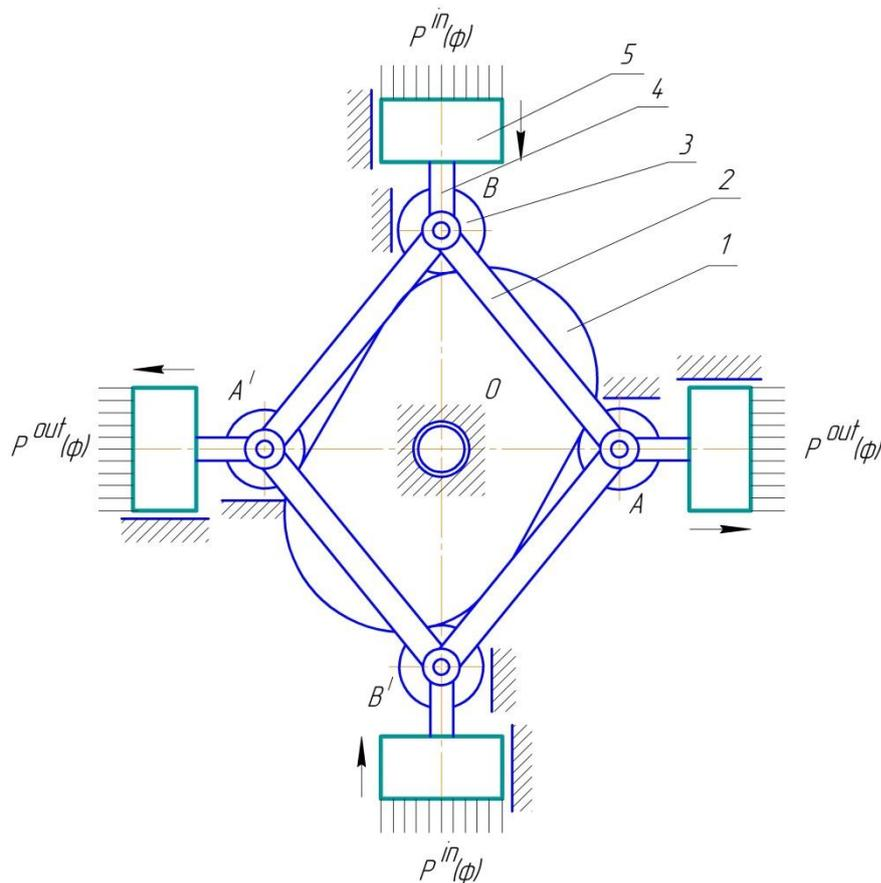
**Figure 2. The structure of the Fairchild mechanism**
