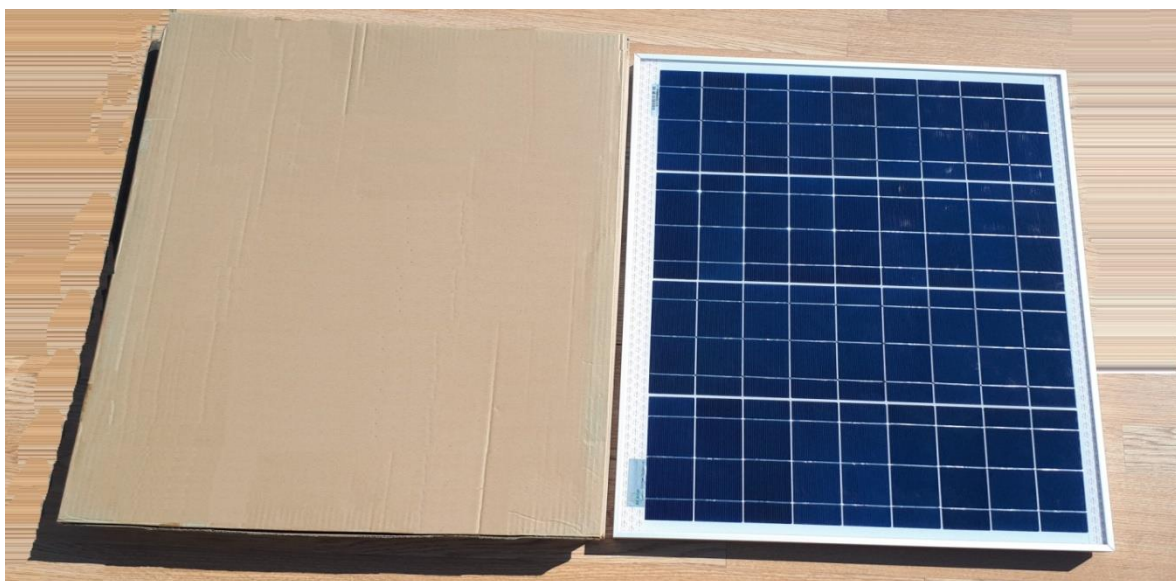
Fig. 1 Photovoltaic batteries selected for the experiment: 1- FEB with a closed surface, 2 - FEB with an open surface.
